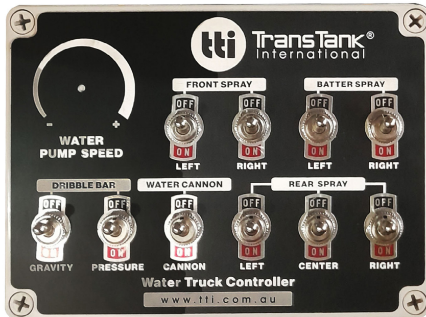
Figure 3 – In-cab Control Panel – Hydraulic Pump Unit
