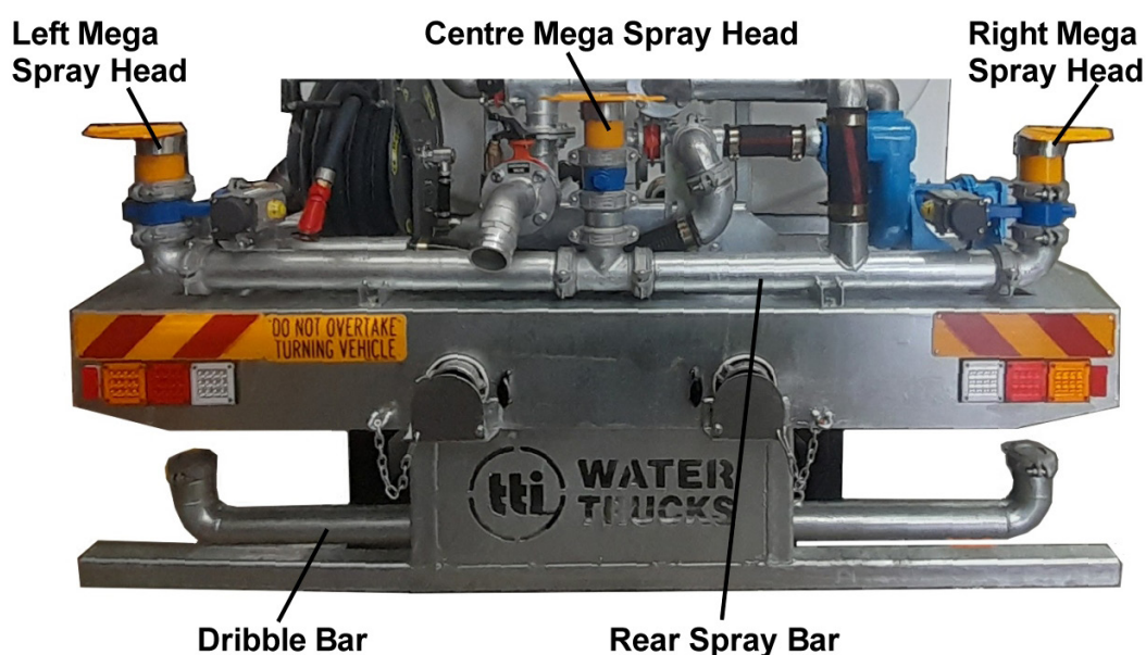
Figure 9 – Rear Spray Bar and Dribble Bar
