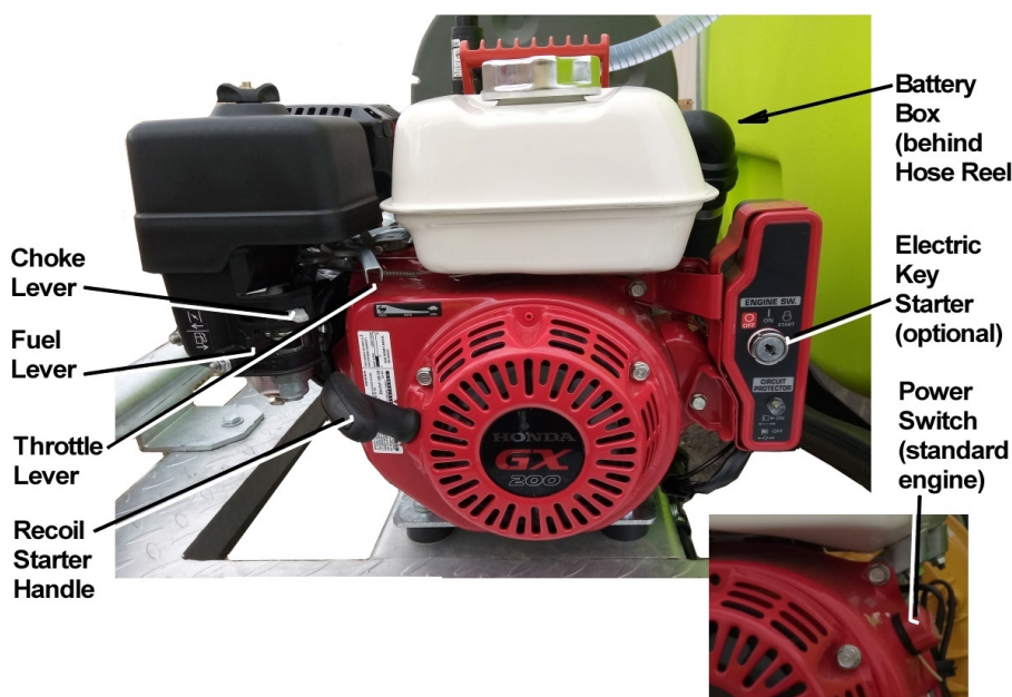
Figure 6 – Petrol Engine Start-up Procedure
