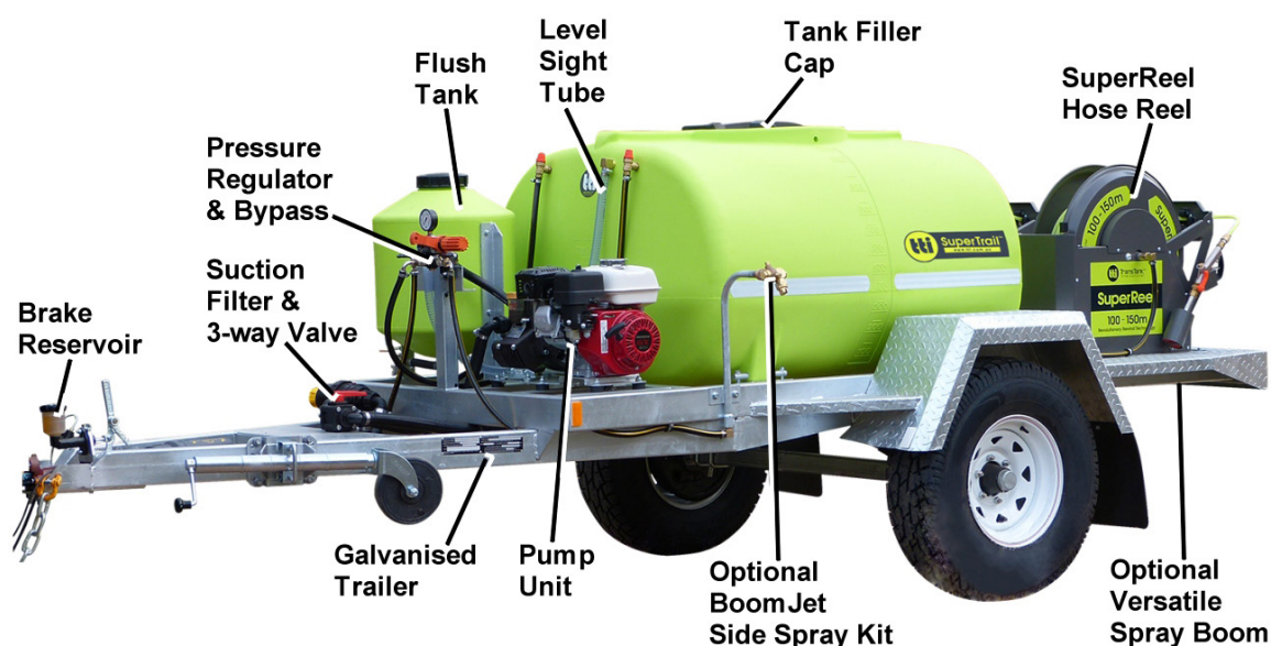
Figure 1 – Component Identification – SuperTrail with side-mounted BoomJet nozzle option
