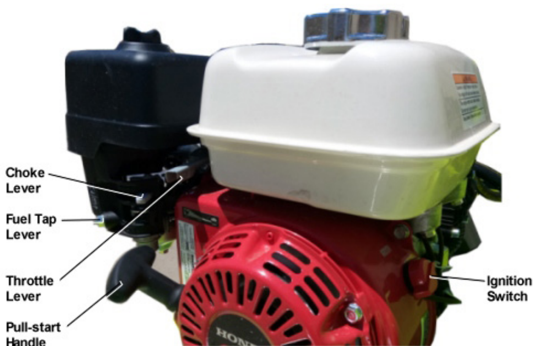
Figure 4 – Petrol Pump Details
