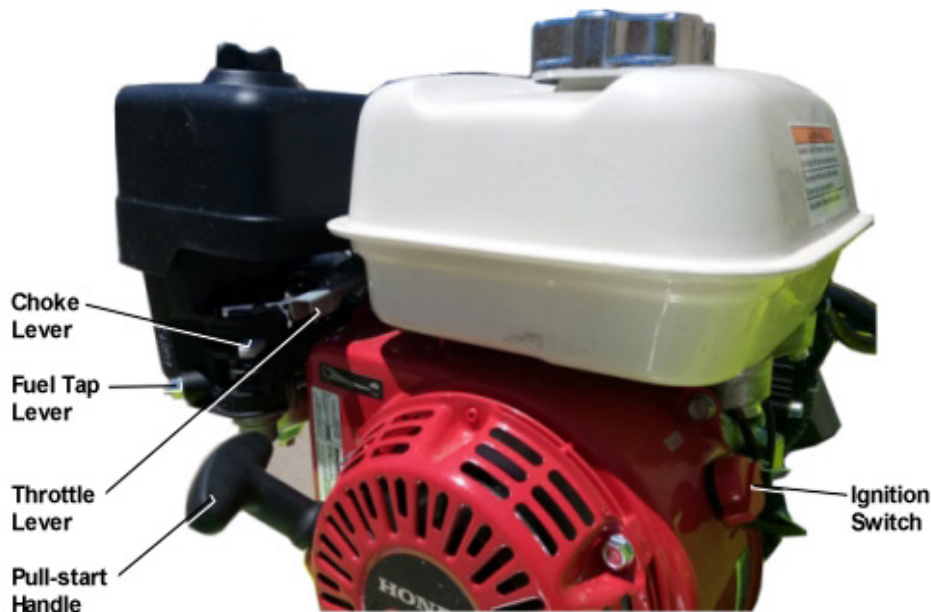
Figure 8 – Petrol Pump Details (GX35 shown, GX200 similar)
