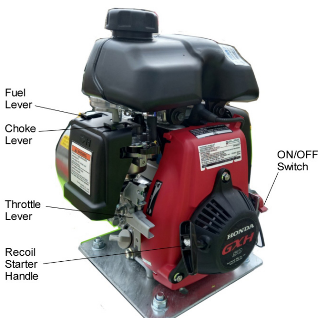
Figure 7 – Petrol Engine Start-up Procedure
